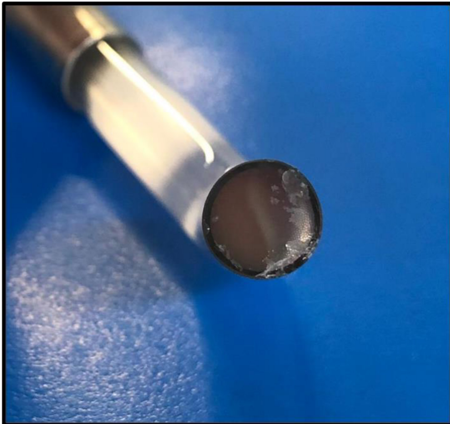
Figure 8 Polymerized composite resin adhered to the surface of a unit tip.
