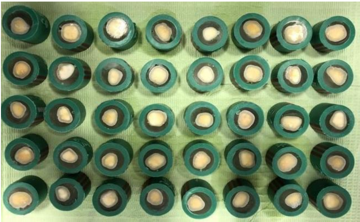
Fig. 1. Standardized pieces embedded in PPL tubes.
