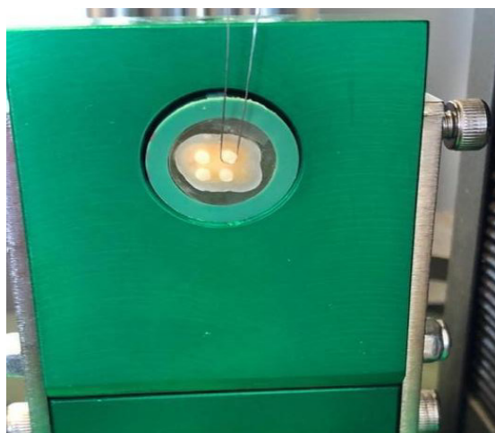
Fig. 2: Universal testing machine performing micro-shear mechanical test.
